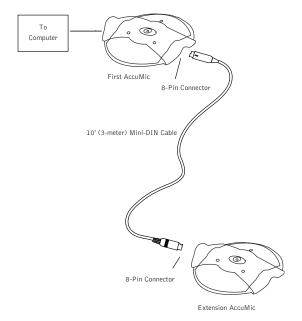
Figure 7. Connecting an AccuMic PC Extension Mic
